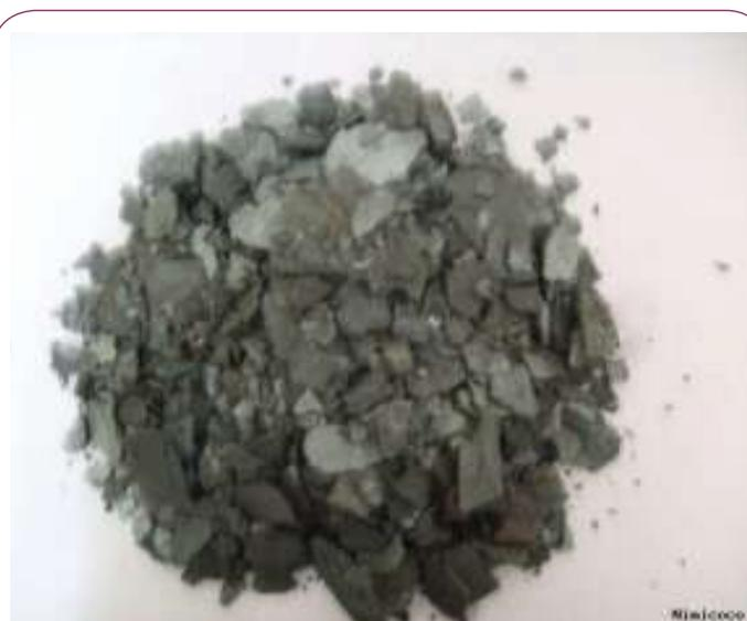
**Figure 1** Photograph of Rolling mill scales. (Composed of 69-72% iron oxides, 20%oil and 10%water).
